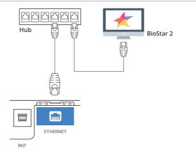
CoreStation has automatic MDI/MDI-X function, so it can be connected to a PC directly using a normal type CAT-5e cable.
